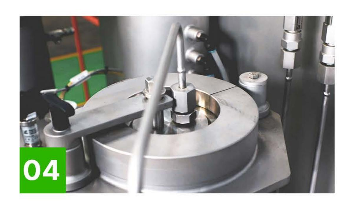
Unique Extractor Closure Design for rapid batch changeovers with minimal interruption
