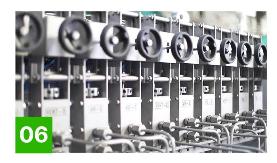
Proprietary Changeover Valves for quick changeovers and isolations, even at high pressures
